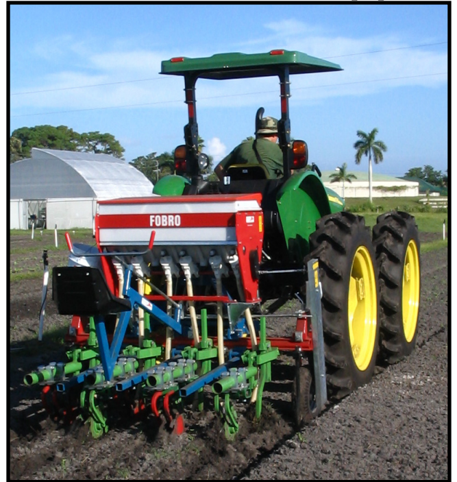
Attached to the back of our high crop tractor is a Star Hoe. This implement does wonders for us - everything from cultivating to fertilizing. Here you can see the machinery incorporating organic fertilizer into the soil before a planting at the first of the season.
